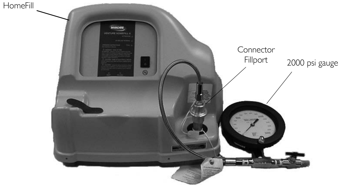
FIGURE 13.3 HomeFill 2000 psi Switch/P.C.B. Shut Down Test
