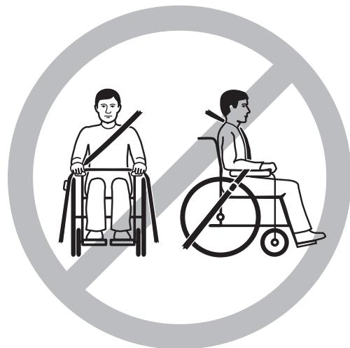
Incorrect placement of belt
