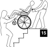
**3.** The wheelchair must not be lowered until the last step has been negotiated and until the chair is clear of the stairs.
