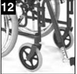
Force the air out the the inner tube by pressing valve A. Stretch the outer case on the rim. Repair or replace the inner tube. Put the inner tube back in place. Reposition the outer case on the rim. Re-inflate the tyre to specified pressure.
