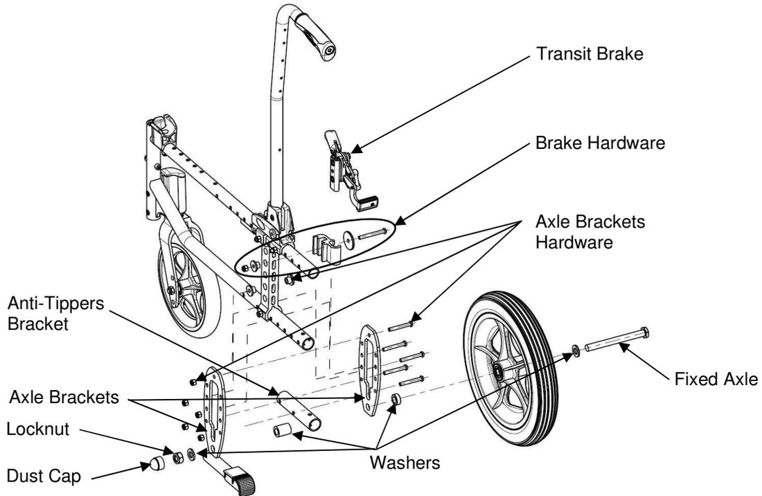
**FIGURE 5.1** Removing/Installing Rear Wheels
