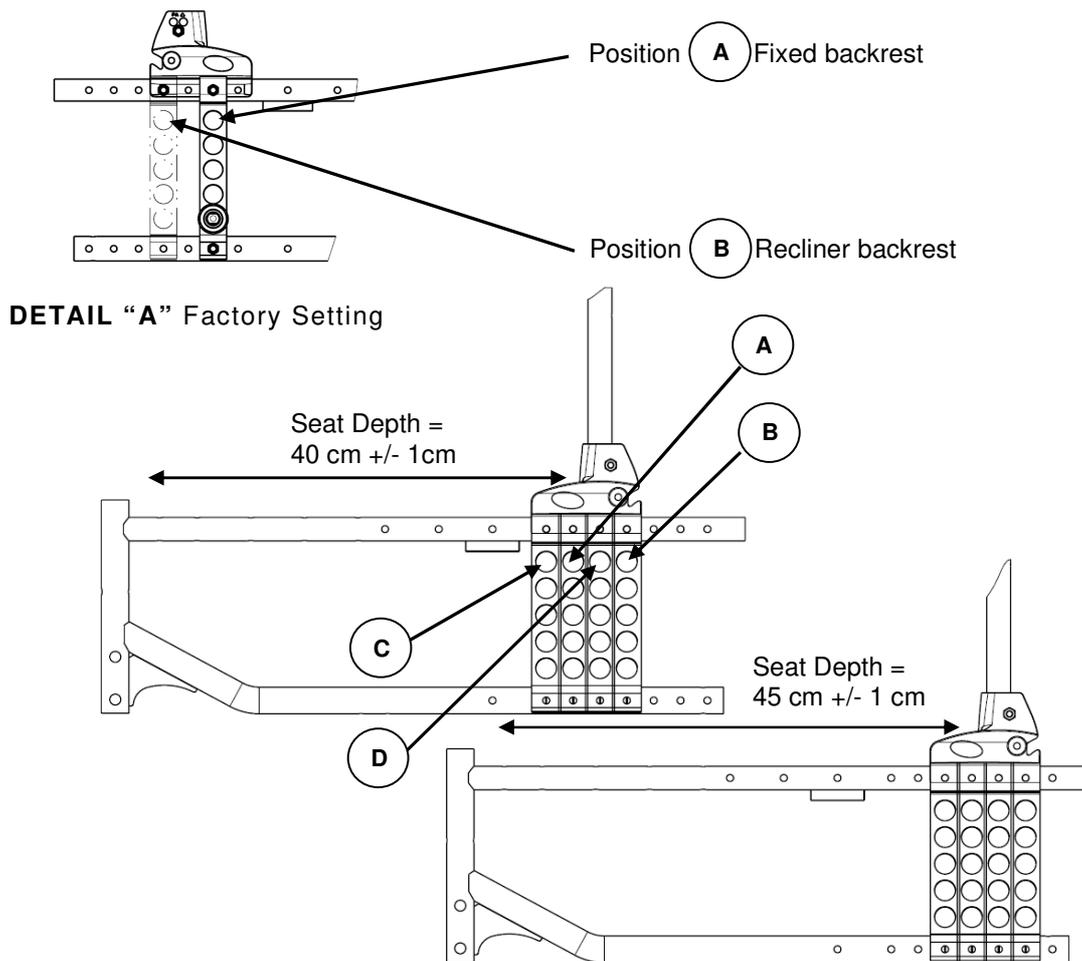
**FIGURE 5.6** 4 Possible Positions of Wheel Plate
