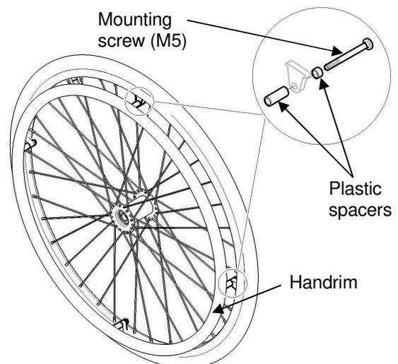
**FIGURE 5.4** Replacing Handrims
