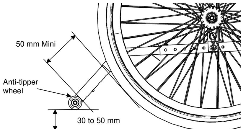
**FIGURE 9.3** Adjusting Anti-Tippers
