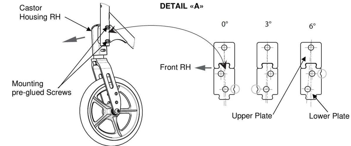
FIGURE 5.11 Adjusting Castor Angle (Castor housing Light)
