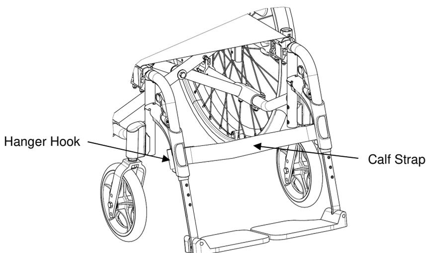
**FIGURE 2.3** Installing Calf Strap
