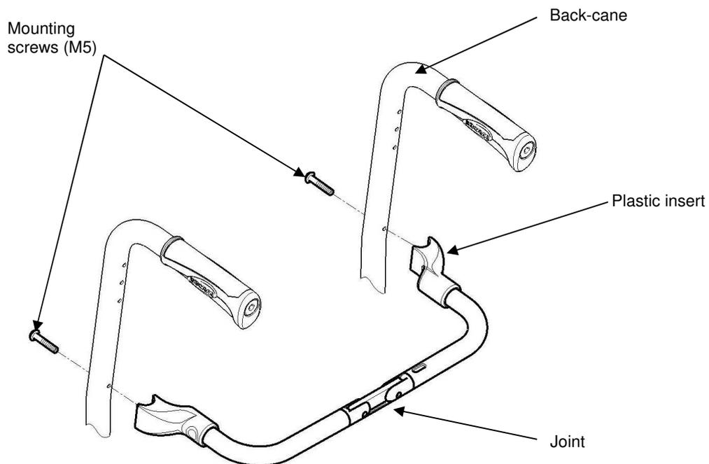
**FIGURE 4.13** Installing/Removing the Folding Back Brace
