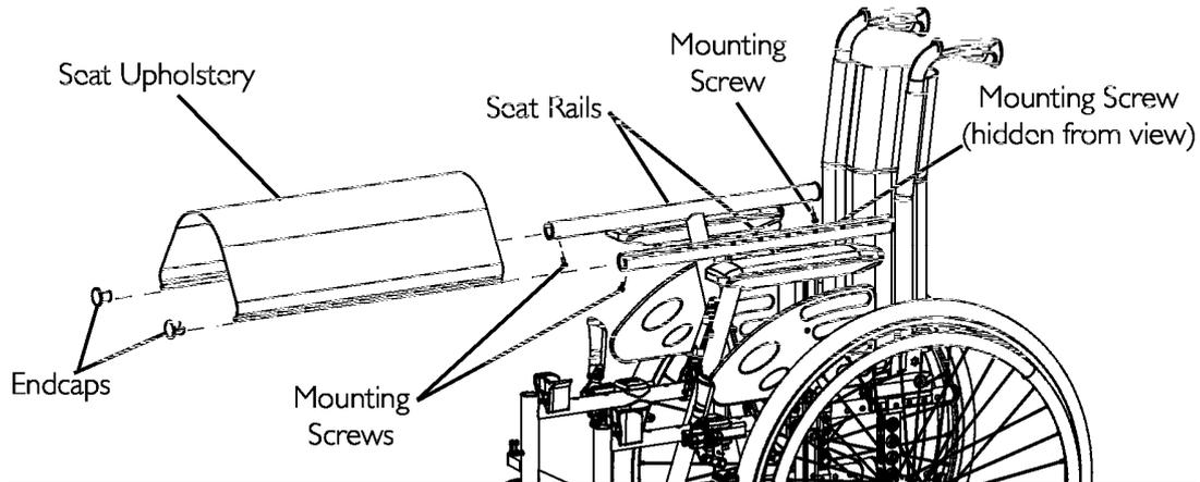
**FIGURE 4.2** Removing/Installing Seat Upholstery
