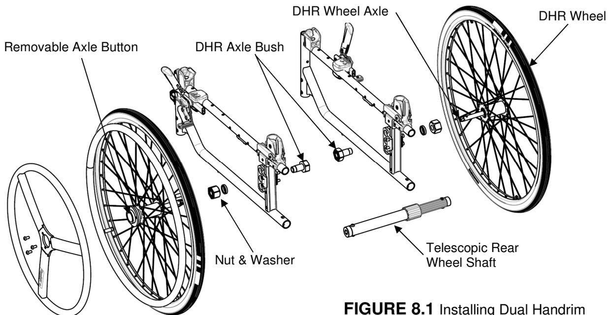
**FIGURE 8.1** Installing Dual Handrim
