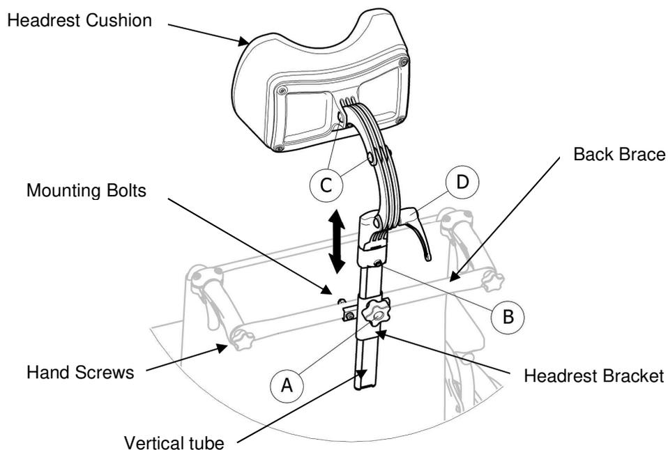
**FIGURE 8.2** Installing Headrest
